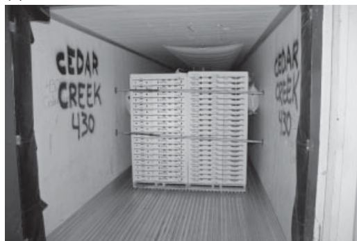
Figure 9.4 (a) After palletisation is complete, the pallets are moved to a fumigation chamber for immediate SO 2 treatment, to a forced-air cooler or fumigation or to a forced-air cooler where fumigation is done at the end of the day's packing. (b) After cooling is completed, the pallets are moved to a storage room to await transport. (c) During transportation, a central loading technique is utilized to maintain cold temperature during the transportation period.
