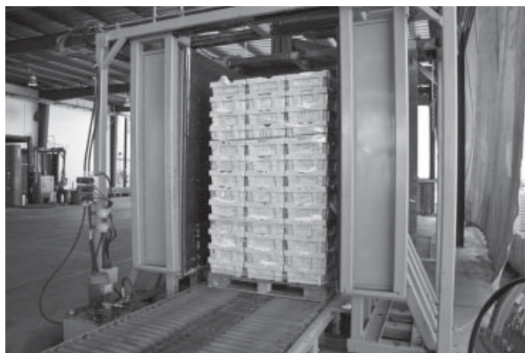
Figure 9.3 Loaded pallets coming from the field often pass through a "pallet squeeze," a device that straightens and tightens the stacks of containers. These pallet loads are unitized, usually by strapping or netting.
