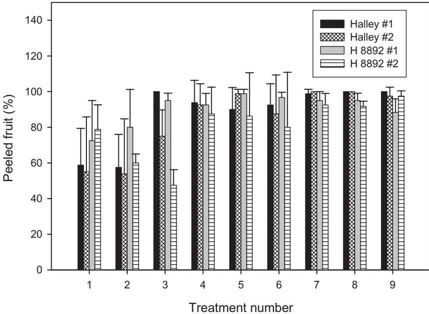
FIG. 1. STEAM AND VACUUM PEELING OF TOMATO cv. HALLEY 3155 AND H 8892
