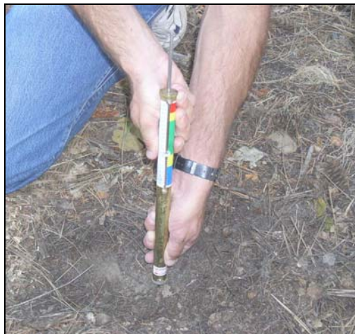
Figure 1 Lang Penetrometer used to measure soil resistance to penetration.
